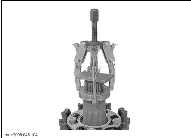
2. Remove the bearing flange.
