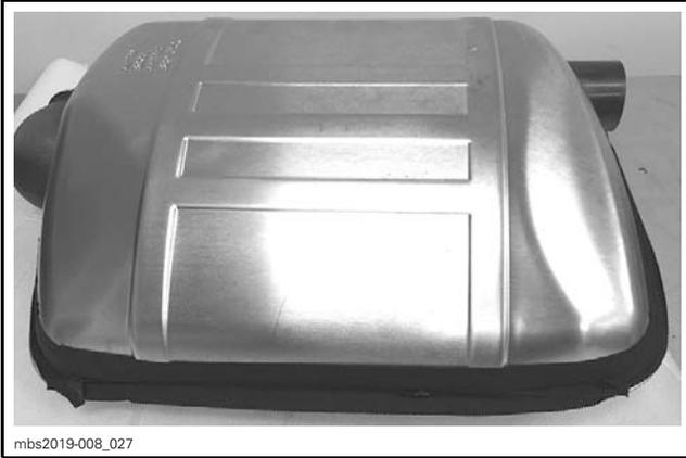
13. Using a steel head hammer, fold up deflector edges up against LH deflector sides, after working around the muffler perimeter, remove the protective tape.
