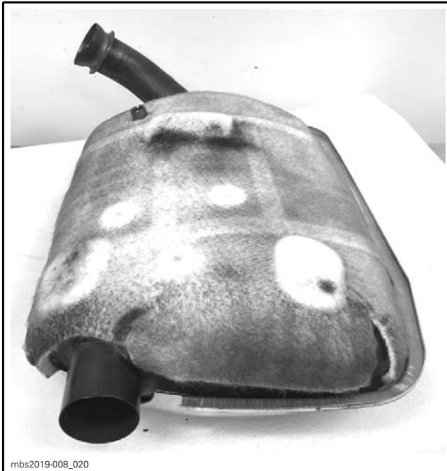
10. Start by folding the RH deflector edge onto LH deflector edge at an approximate 60° angle using a nylon head hammer all around the muffler perimeter.
