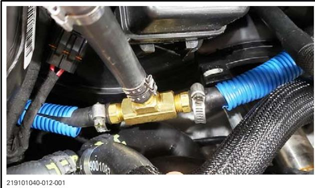
5. Install the pressure gauge on the T fitting tool.
