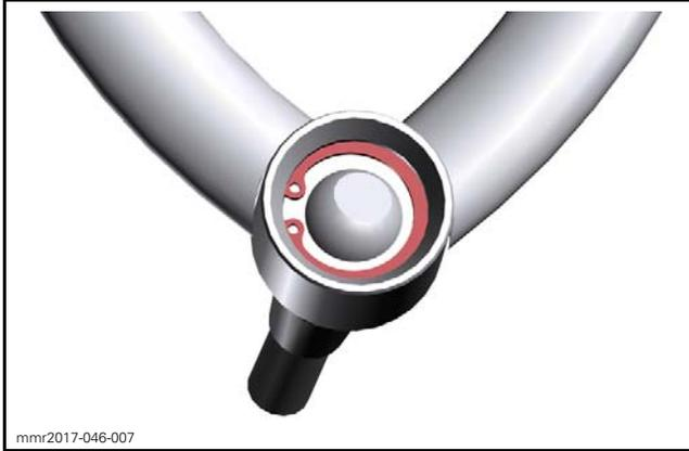
3. Press ball joint out of the suspension arm.
