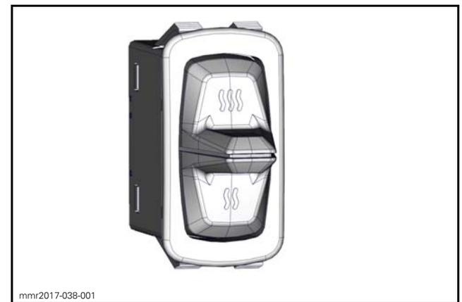
HEATER SWITCH - MODELS WITH CONSOLE SWITCH
