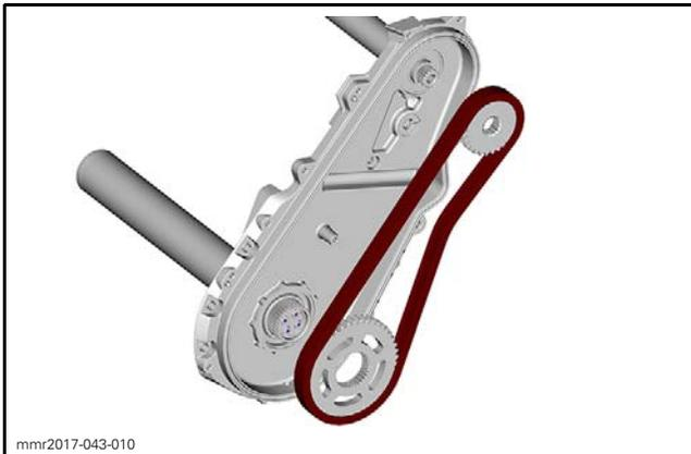
4. Remove the countershaft spacer.
