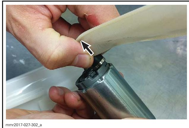
6. Discard inlet fuel pump filter and steel ring.
