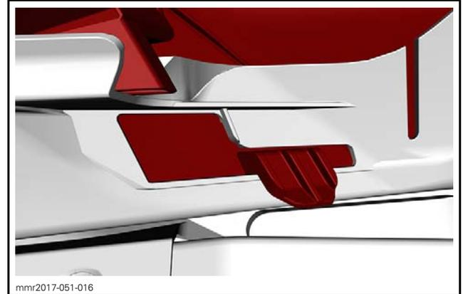
Ensure to connect the air intake hose.
