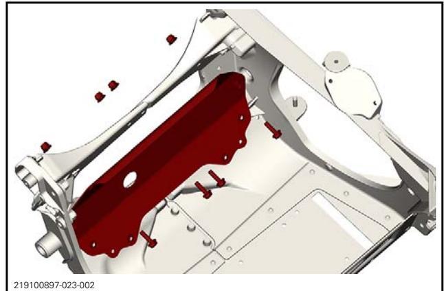
Remove HUCK rivets as per the procedure in this subsection.
