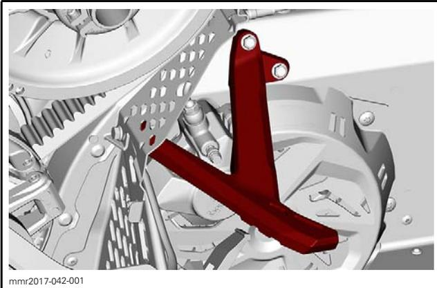
6. Remove the disc brake protective cover.
