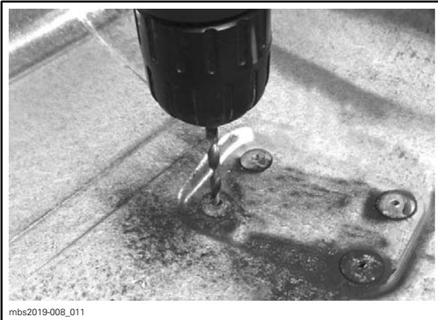
6. Put a clean rag on your work bench for protection, reinstall all three brackets on LH deflector using new rivets.
