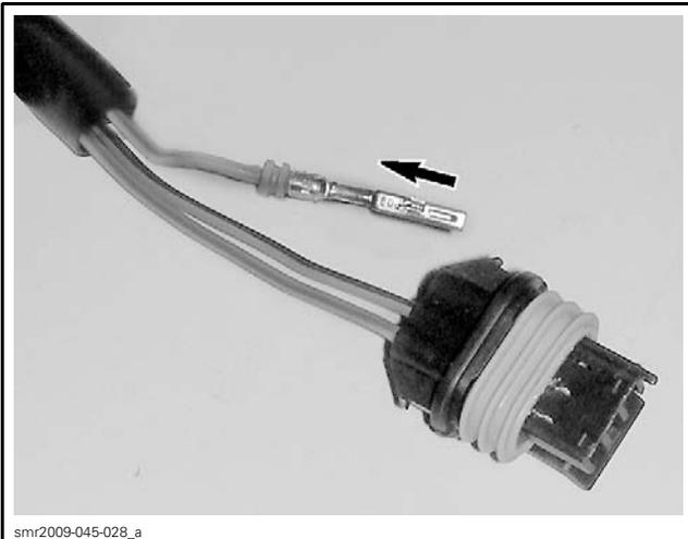
**NOTICE** Before installing terminals in the connectors, ensure all terminals are properly crimped on the wires. After installation of the wire terminals in the connectors, ensure they are properly locked by gently pushing on them as if to extract them.
