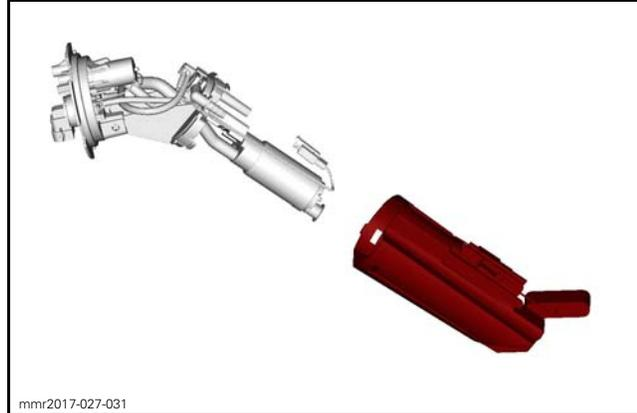
**NOTICE** To avoid damaging wires, Pull the reservoir carefully and do not let reservoir hang by wires.
