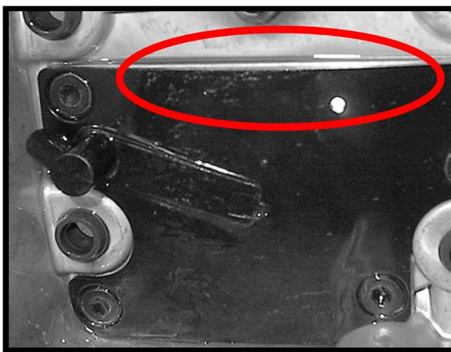
The correct way to install the breather subassembly is to lubricate the bottom O-ring (A) with general purpose grease and twist the breather subassembly back and forth until the breather is properly seated into the labyrinth plate (B), then tighten the (2) breather bolts (C) to specification.
