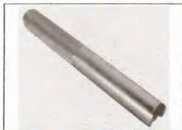
Floating piston support P/N 529 035 903 Recommended ZX X 440
