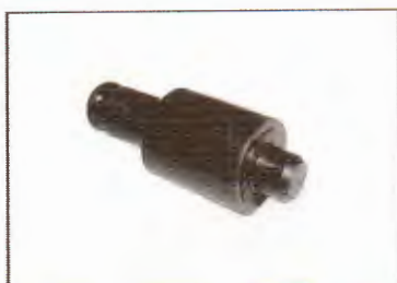
Oil seal pusher P/N 529 036 210 Recommended 602 ACE
