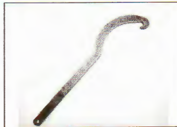
Drive pulley holder (CVT) P/N 529 006 400 Recommended
