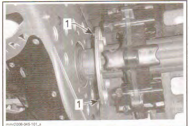
1. Bearing flange locking tabs
