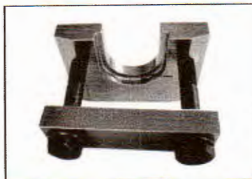
Ball joint extractor P/N 529 035 827 Mandatory REV, RT
