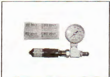
Gas fill tool kit P/N 503 190 102 Recommended T/A shocks To be used with P/N 529035570. Spare needle P/N 529035930.
