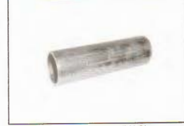
Crankshaft bearing installer (MAG) P/N 529 035 980 Recommended 552, 593HO, 693, 793 engines
